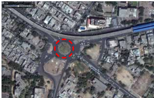
Time Line year: 2010 The roundabout was re-structured by adding another arm from Dr. K.S. Krishnan Marg. To manage the increased traffic and multiple traffic islands the roundabout was signalled.
